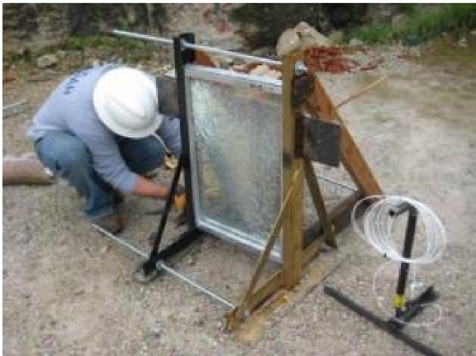
An engineer from the University of Missouri studies the glass pane after a test explosion. (Credit: DHS S&T)
